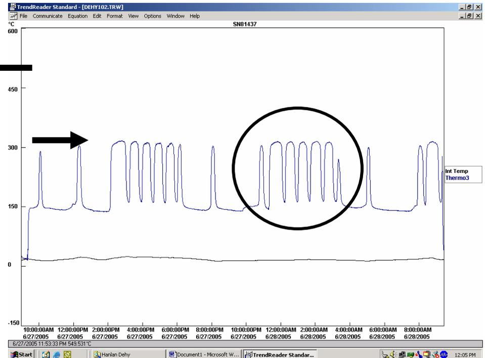
**Duty Cycle to the Extreme** - This is the consequence of an **extremely low main burner duty cycle**, only the pilot ran, **condensing moisture in "Products of Combustion"**. Water accumulates and freezes at the flame cell as it tries to drain out. Level rises until even the pilot is extinguished! This is a concern for oversized heaters, more common a problem than we accept.
